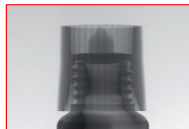
Sample is too far away from the X-ray source, low magnification
