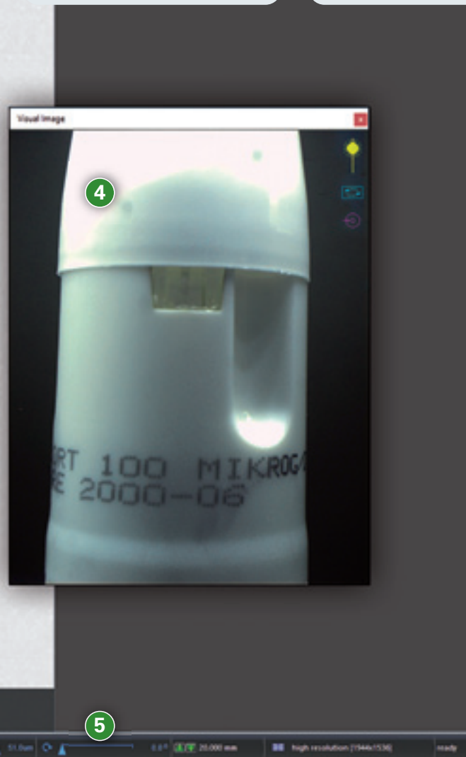
Overview of the SKYSCAN 1275 control software window Inhaler, 40 \mu m voxel size, 100 kV, 1 mm Cu filter, 972 x 768 px
