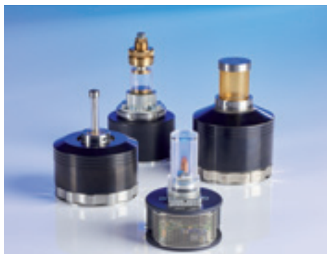
Various sample holders and in-situ stages
