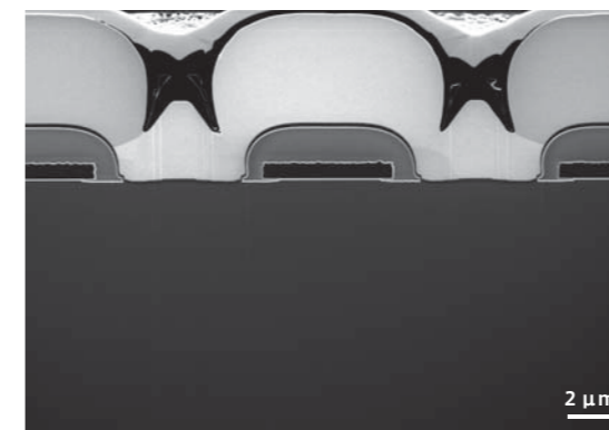
Before ion milling (FIB fabricated surface) 2 µm
