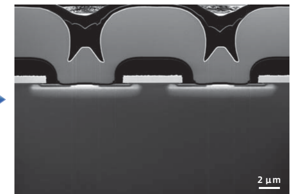
After ion milling (FIB fabricated & Ion milling) 2 µm Specimen: silicon carbide (SiC) power device
