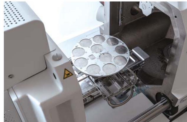
Example of 47 mm diameter X 11 Specimen holder (SU3900SE)
