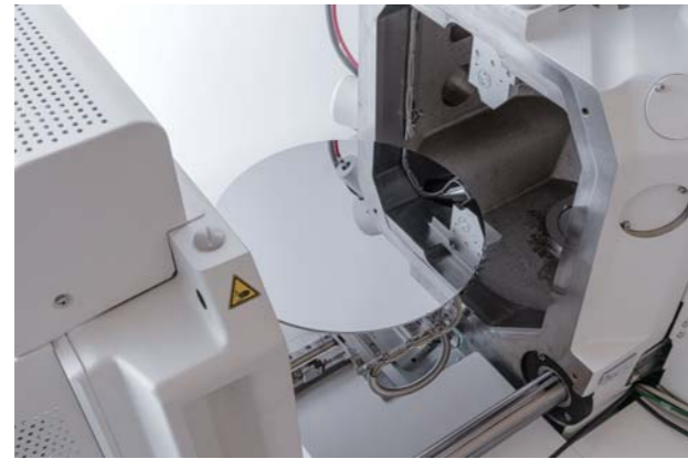
Example with 300 mm diameter wafer loaded (SU3900SE)
