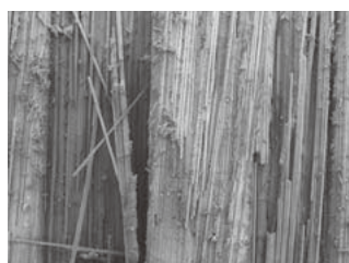
Low accelerating voltage SE image Sample: CFRP
